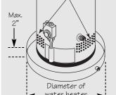
The pan must not restrict air flow to the combustion air inlet openings (perforation openings) located around the lower perimeter of the water heater.
